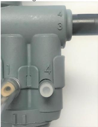
6. Install four 5.5" pre-cut lengths of tubing onto the four hose barb ports of the QDV valve. Insert four in-line check valves, with arrows pointing toward the QDV valve, into the open ends of the pre-cut lengths of tubing.
